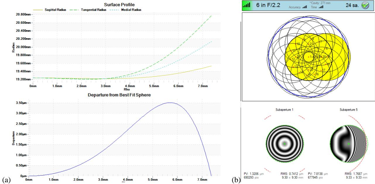
Figure 2: Characteristics of S13 prior to optimization (a) local radius of curvature and departure plots and (b) lattice design
