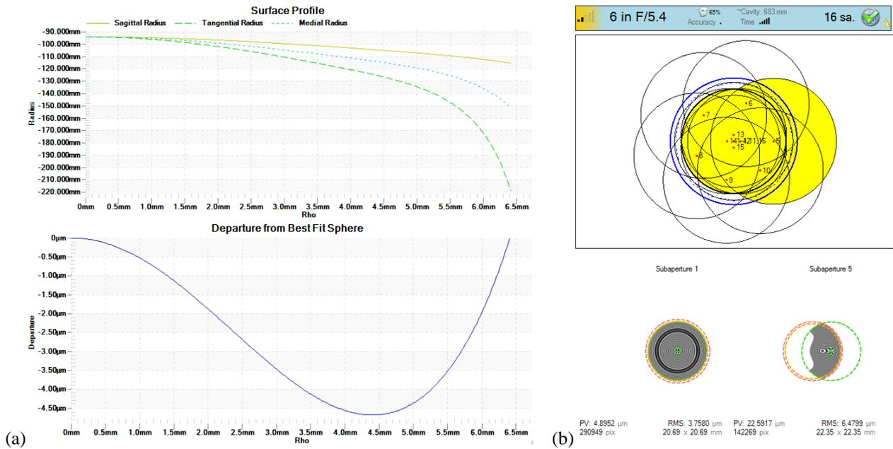
Figure 5: Characteristics of S14 after optimization (a) local radius of curvature and departure plots and (b) lattice design
