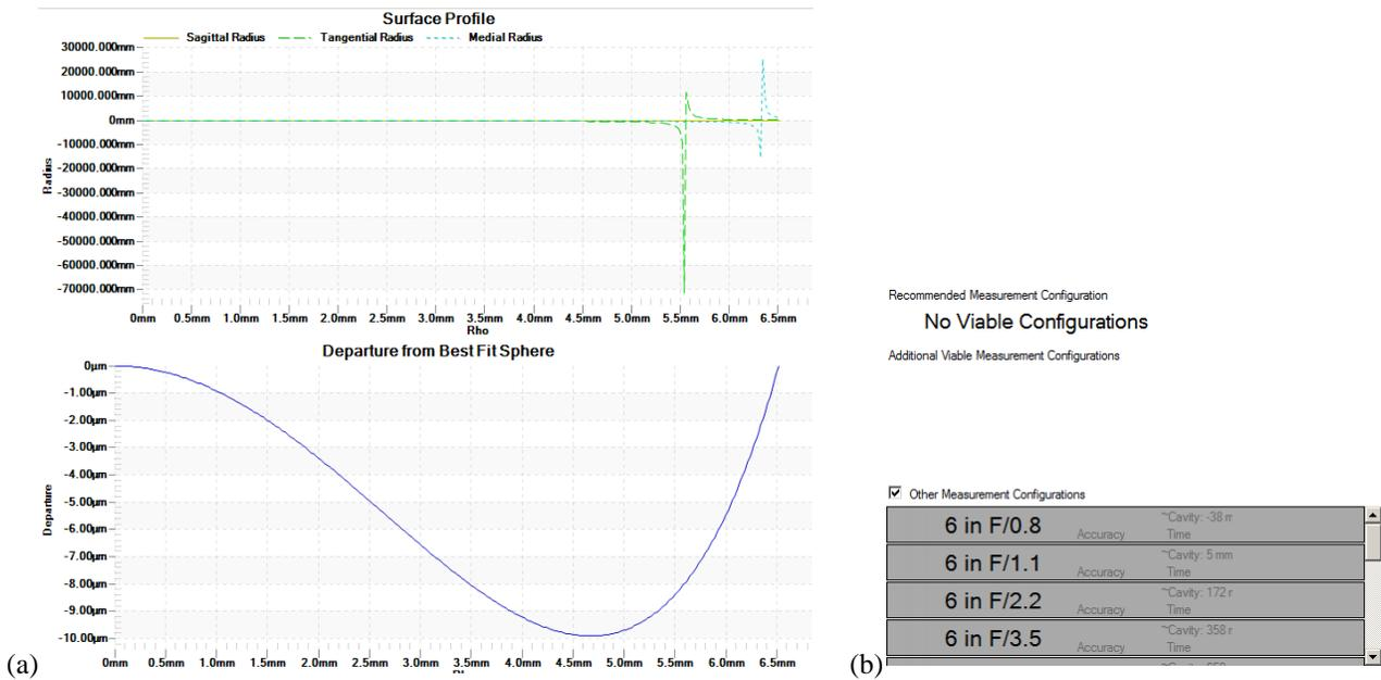
Figure 3: Characteristics of S14 prior to optimization (a) local radius of curvature and departure plots and (b) lattice design. No SSI lattice can be designed despite the relatively mild departure, due to the inflection point inside its clear aperture.
