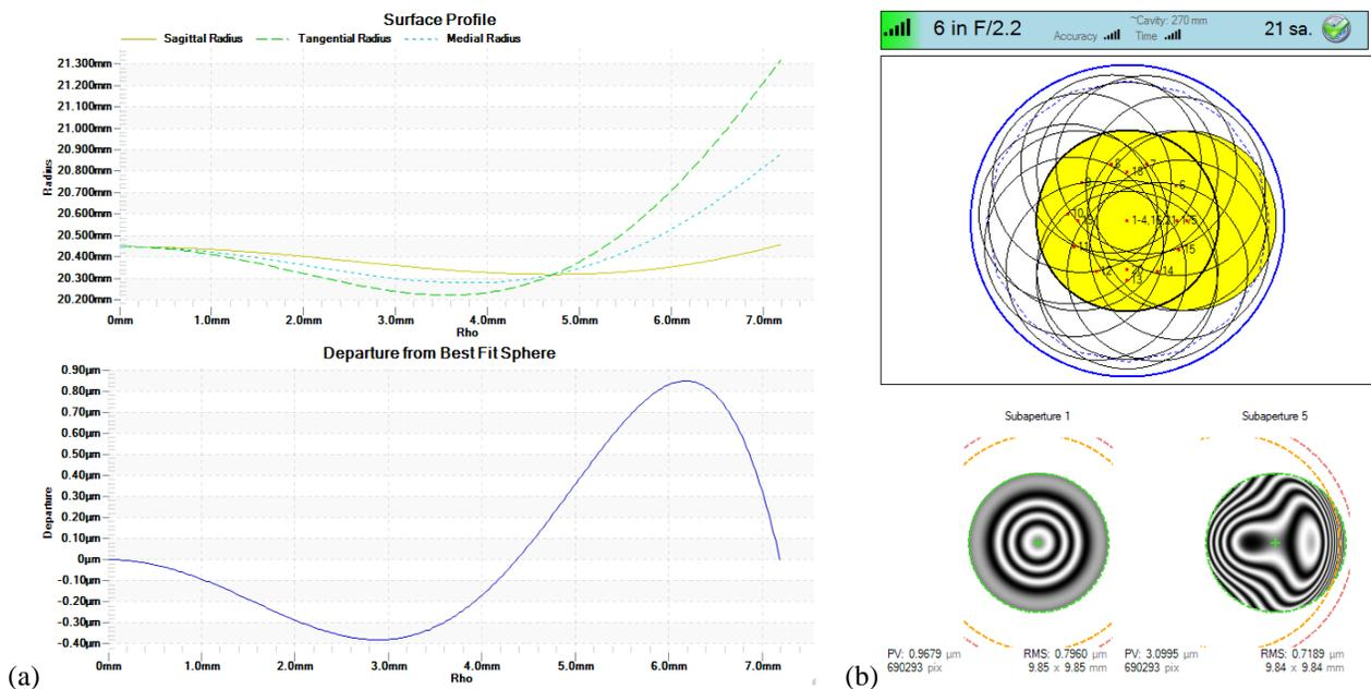
Figure 4: Characteristics of S13 after optimization (a) local radius of curvature and departure plots and (b) lattice design
