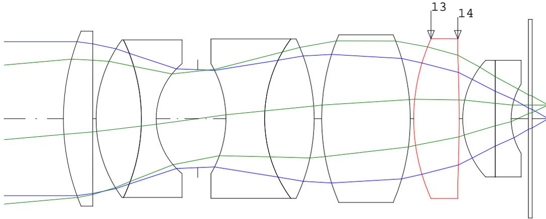
Figure 1: Cross section diagram of the nominal design of our microscope objective optimization example. The two aspheric surfaces are labeled 13 and 14.
