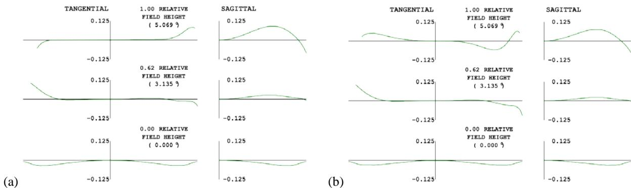
Figure 6: Wavefront plots (in waves 632.8 nm) for the system with 15.5 mm focal length,  $\pm 5^\circ$  field of view, and 0.5 NA: (a) initial (b) after SSI-A penalty function reoptimization – the average rms over the field points changed from 0.0214 to 0.0237 waves (an insignificant amount for this design)
